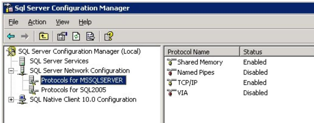
3. Verify that the **TCP/IP** Protocol is "Enabled". If it is not enabled, double-click on the protocol and change its properties to enabled. You will receive a warning that the service will need to be stopped and restarted:
